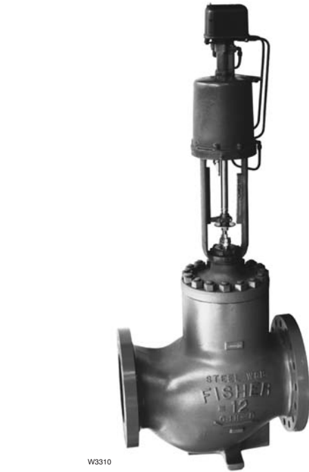
Figure 9A-5. The Design EWNT-1 is typical of globe valves used for DALC service. Flow resistance is minimal at high loads and cavitation protection is provided for low load operation and startup.
