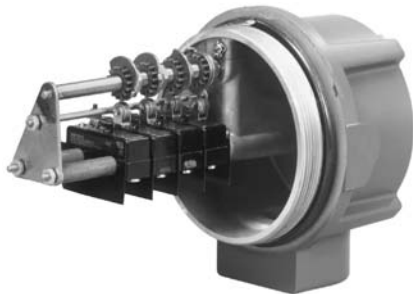
Figure 2-14. Limit switches are a common actuator accessory. This unit can accommodate up to six switches and has trip points adjustable to any point in travel.
