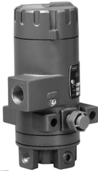
Figure 2-13. Electro-Pneumatic transducers are a common actuator accessory. They take a milliamp signal and produce a proportional pneumatic output. The Type 646 is compact, accurate and has low air consumption.
