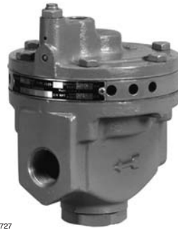
Figure 2-15. On fast control loops, a positioner may not be able to react quickly enough to be of use. In these situations, performance of spring-and-diaphragm actuators can be improved by use of pneumatic boosters such as the Type 2625.
