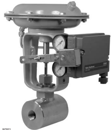
Figure 1-5. Bar stock valves such as this Baumann 24000SB provide economical solutions to small flow requirements. It is capable of pressures to 1500 psi and temperatures to 450 °F. Compact spring and diaphragm actuators complement these small bodies.
