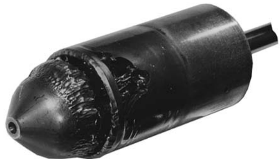
Figure 6-6. The top plug shows the characteristic rough texture of cavitation damage, which differs greatly from the polished appearance of damage due to flashing (lower photo). The two damage mechanisms vary greatly.
