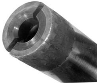
Figure 10-3. End view of the same plug shown in Figure 10-2. Note the light band adjacent to the O.D. and the outside of the plug where the erosion-corrosion damage has occurred. This view also shows how the sample was removed for further evaluation.
