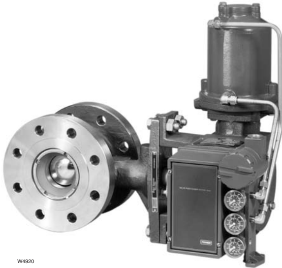
Figure 2-10. The Type 3620JP is an electro-pneumatic positioner that combines the functions of transducer and positioner into one unit. The combustion unit generally is more economical but may not be as flexible as separate units.
