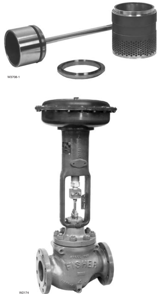
Figure 9A-4. The Design ET with Cavitrol trim is recommended for condensate pump recirculation applications. Its drilled hole trim gives protection from cavitation damage. Tight shutoff is also featured.
