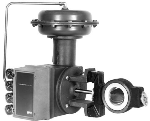
Figure 1-12. Lined butterfly valves offer tight shutoff but are limited to low temperature applications. The liner material keeps the process away from the metal body eliminating many corrosion problems.
