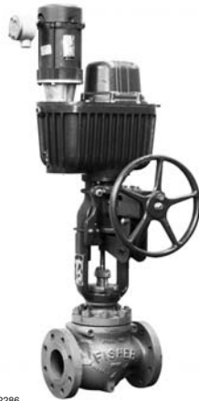
Figure 2-8. The Type 350 is a “self-contained” electro-hydraulic actuator. The single unit incorporates a hydraulic pump and reservoir.
