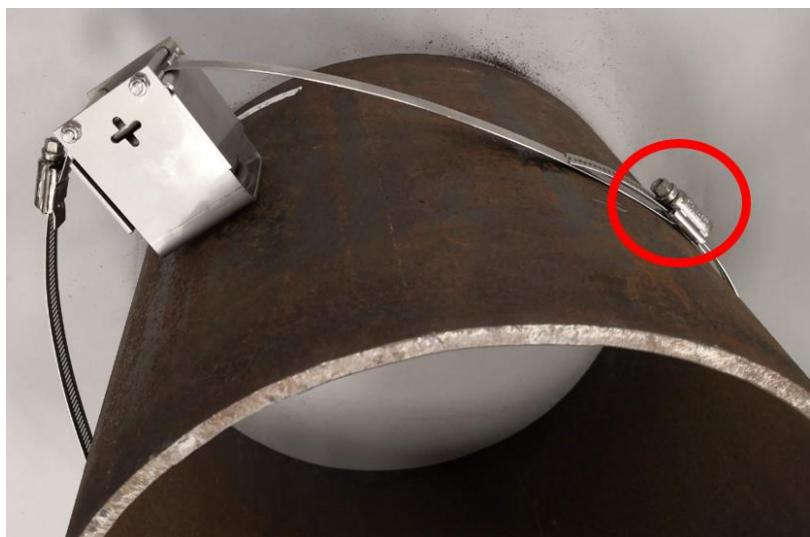
11. Ensure the strap tensioner, strap and sensor(s) are in-line before tightening the worm-screws on the strap tensioner.
