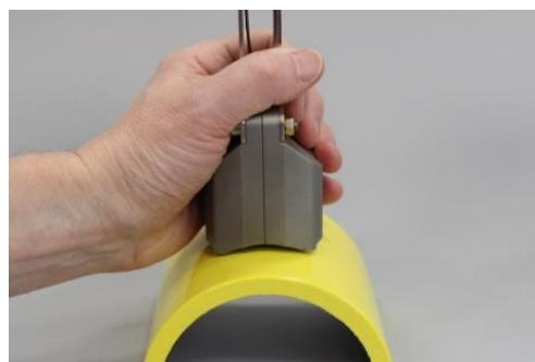
7. Feed the previously cut strap through the strap slot hole of the sensor and around the pipe
