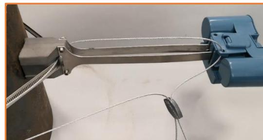
**Note:** The lanyard wire can be released from the 'lock' using the release key.
