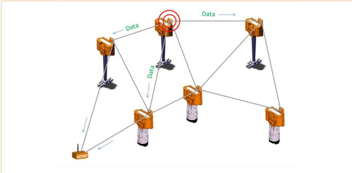
Figure 3. Mesh networking in Permasense WiHART sensors
