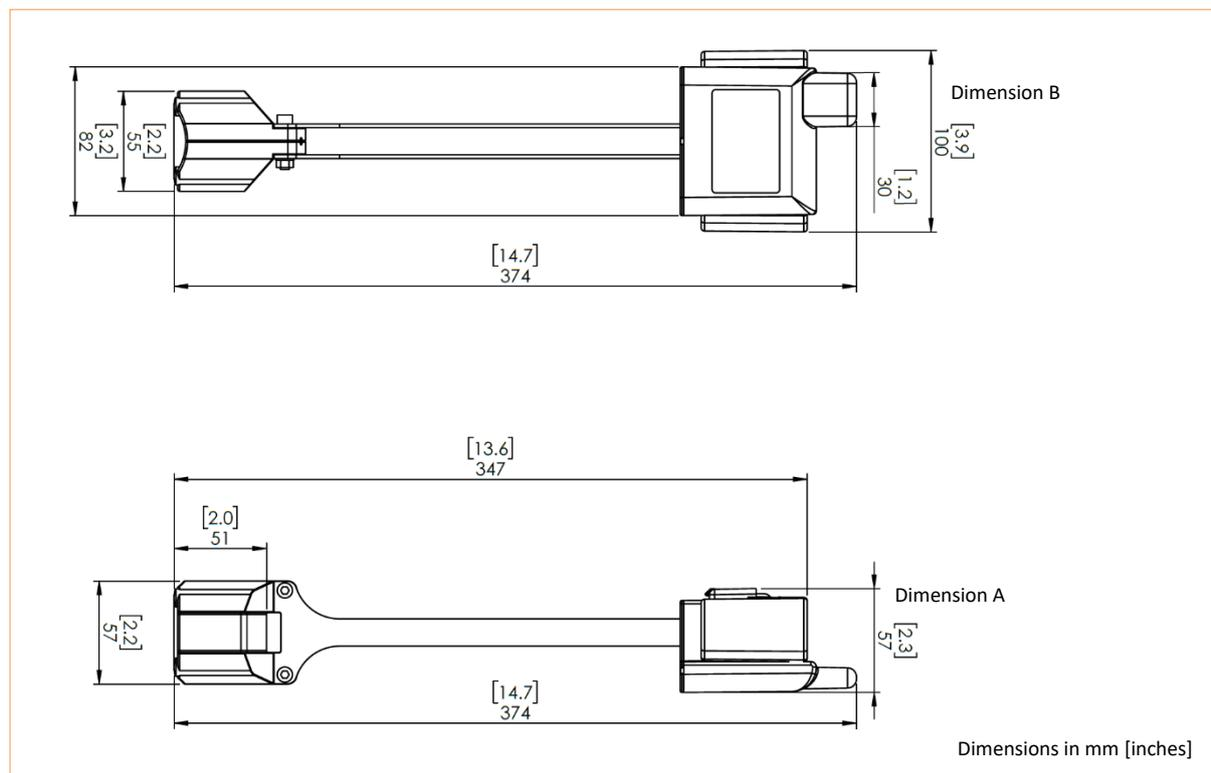
Figure 2. Dimensions of the ET410 sensor, shown with a BPI0E power module
