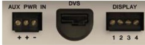
Figure 5-5. Display Connection on Base Unit
