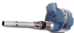
The Rosemount 142 contacting conductivity sensor is a screw in type sensor available with 0.01/cm and 0.1/cm cell constants. Interconnecting cable for wiring between sensor junction box and transmitter is sold separately.
