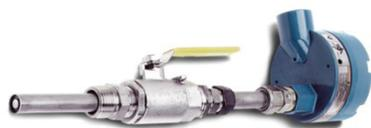
The Rosemount 140 contacting conductivity sensor is a retractable type sensor used to measure conductivity in process liquids having moderately high conductivity. Sensors are available in 0.2/cm and 1.0/cm cell constants. Interconnecting cable and ball valve/retraction assembly must be ordered separately.
